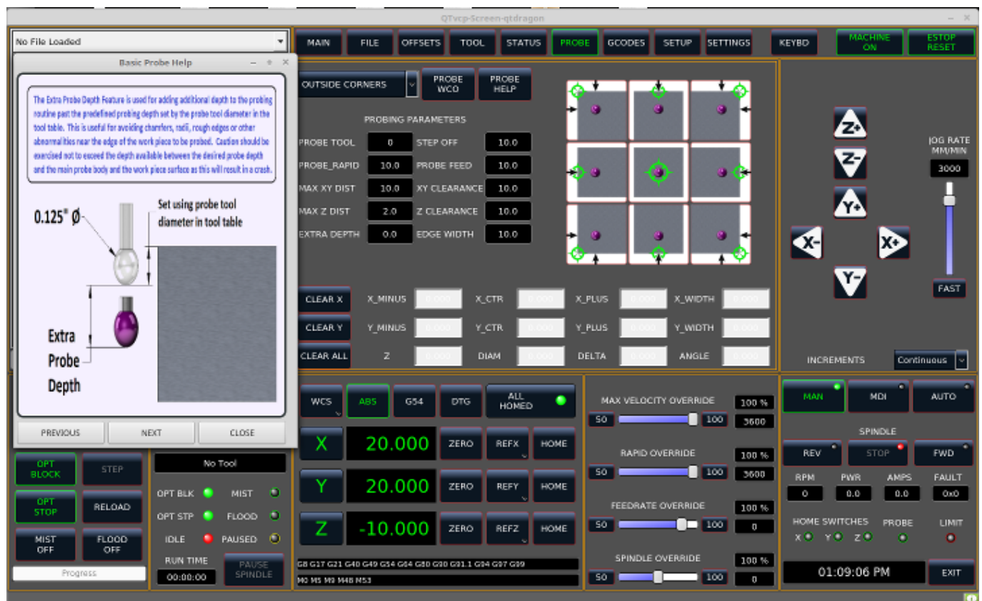
Figure 10.30 – QtDragon - Basic Probe Option
